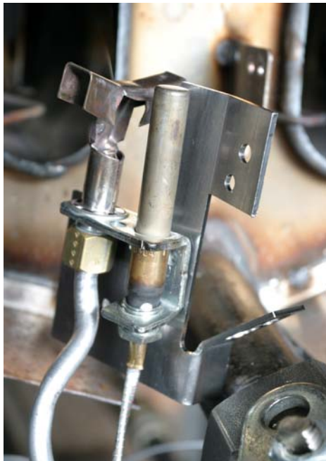
3 - 4: Remove the existing pilot/thermocouple assembly from the bracket on the frypot and attach the assembly, with the provided screw, to the provided bracket, as shown above.
