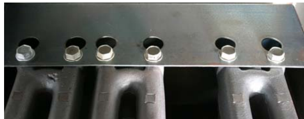
2: The burners are secured by bolts, which are visible when the shield is removed. Loosen the bolts and lift up the burners to remove.
