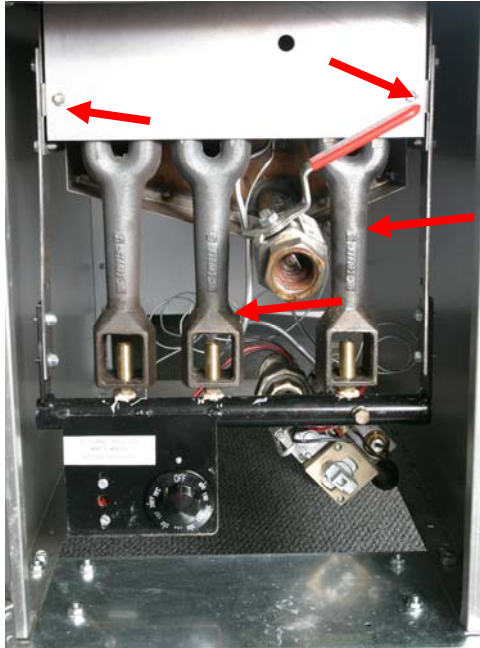
1: The cabinet is shown prior to installation. The shield in front of the burners must be removed along with two burners.
